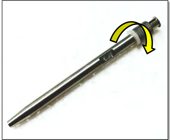
Twist Stinger Needle into Luer Fitting
