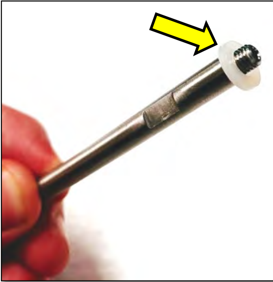
Seat SMC Washer onto Stinger Needle
