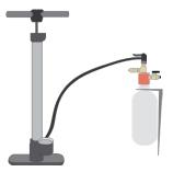
Once the bottle and harness are empty of cleaning solution, pressurize the harness with air to flush any remaining fluid into the waste container. Dispose of pesticide wastes and rinsate in accordance with the product label and local, state, and federal regulations.
