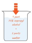
Thoroughly clean the harness connector, pressure relief valve, and other components as needed. It is recommended to remove and soak the harness connector in cleaning solution after heavy use.
