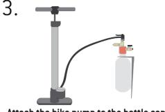
Attach the bike pump to the bottle cap Schrader valve.
