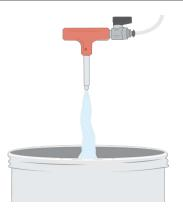
One at a time, open the injection tee valves over a rinsate collection container (such as a bucket with lid or empty injection bottle) to allow cleaning solution to flow through each tip.
